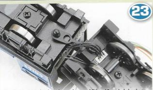
To take the LED wires into the tender, an additional 2mm hole has been drilled in front of the first tender axle. The hole is as close to the wheel as possible to ensure the wires don't get trapped by the tender body.
