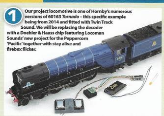
To begin, the locomotive and tender need to be separated to ensure we don't damage any of the model's details during handling. The tender drawbar simply unhooks, but we also need to disconnect the four-wire plug from the tender chassis. We use Hornby's X6468 plug extractor tool to ensure we don't put any strain on
