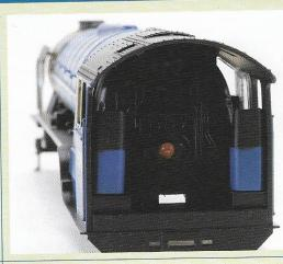
The hole in the firehole door is a perfect fit for the orange LED which peeks through into the cab area. Once a crew has been installed, the LED won't be visible, but its
