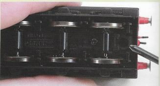
A single crosshead screw at the bottom of this well holds the tender body in place. Once you have removed it, keep it safe for refitting at the end of the project.
