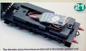
The decoder wires have been positioned in the tender speaker well and the decoder has been positioned on top of the socket completing this phase of the installation. At this point you could refit the body or continue with our guide to add a stay alive.
