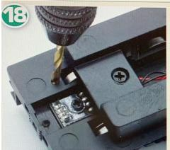
To make an opening for the new speaker wires to enter the tender, a 2mm hole is made through the chassis using a pin vice. Don't be tempted to use a power drill for this a handheld pin vice gives much greater control.
