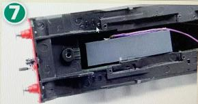
Removal of the leading section of weight from the chassis, held in place with a single screw, makes a large 45mm long space available in the smokebox and boiler – the perfect place to install a Rail Exclusive 40mm x 20mm x 10mm 'Boom Box' speaker.
