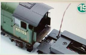
The tender has now been reconnected and the speaker wires fed through the new hole. They are longer than necessary, but can be trimmed to length.
