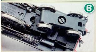
In previous 'A3' sound installations, we have cut away the coal space to make more space for a speaker, but in this case we looked to the locomotive for a new location. The body is held in place with a single crosshead screw located above the front bogie.
