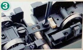
Next, the slotted screw on the tender can be removed allowing the drawbar to be released.
