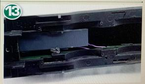
The speaker is fixed in position in the boiler with Black Tack – a semipermanent but strong adhesive. The speaker wires have been positioned along the side of the boiler barrel out of the way of the mechanism.
